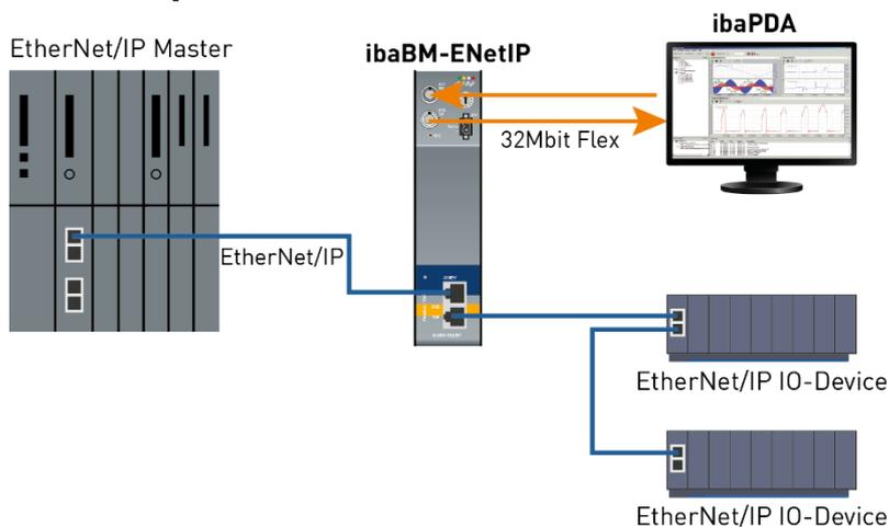
In the above example, the TAP interface is used for acquiring and analyzing the transferred data without interferences. It does not have to be integrated into the configuration of the EtherNet/IP scanner (master).
