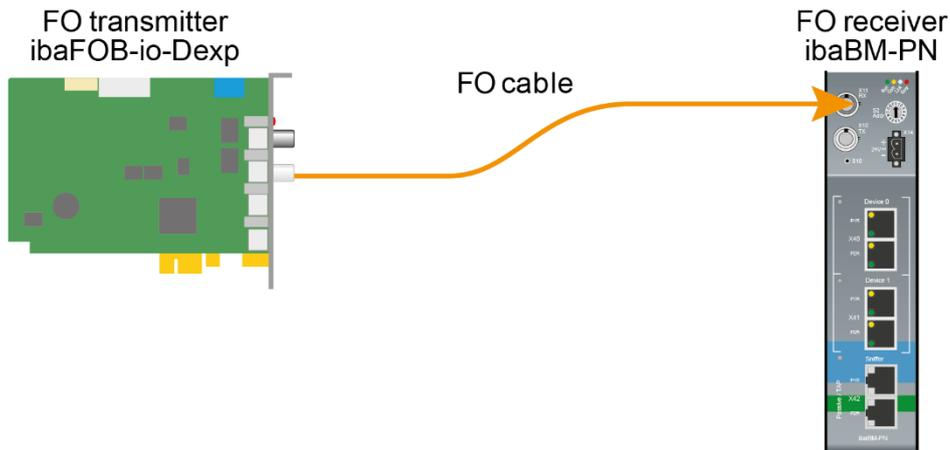
The example refers to a point-to-point connection with an FO cable of type 62.5/125  $\mu\text{m}$ . The light wavelength used is 850 nm.
