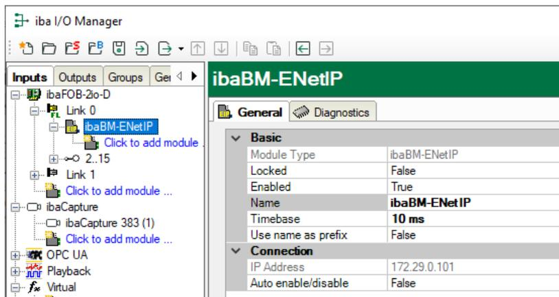
8. Add a module under the ibaBM-ENetIP device. Click with the right mouse-button on the ibaBM-ENetIP device and select "Add module" and the module "EtherNet/IP sniffer" from the list.
