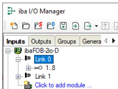
5. Click with the right mouse button on the link and select "Autodetect". The device is identified automatically and shown in the module tree. Depending on the Flex address (switch S2), the device appears at the respective address position 1-15.
