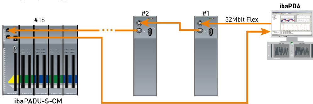
In a ring with 32Mbit Flex protocol, up to 15 devices can be connected. In the ring, all configuration and process data are transmitted.
