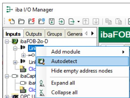
6. Optionally, you can also add the device manually. In this case select "Add module - ibaBM-ENetIP" in the context menu.
