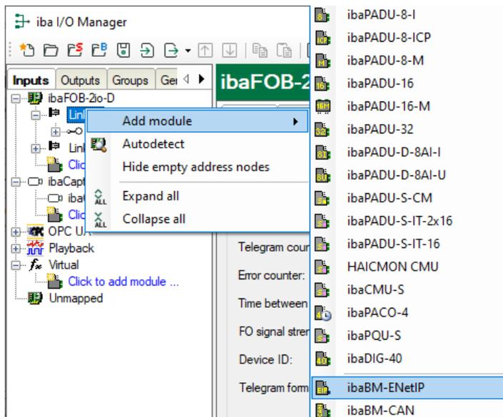
According to the selected Flex address (switch S2), the device has to be dragged to the correct address position using drag & drop.
